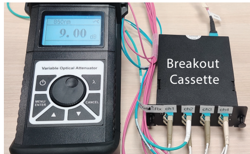
Figure 5.9: Variable Optical Attenuator (VOA) setup used in the motivation and evaluation experiments.
